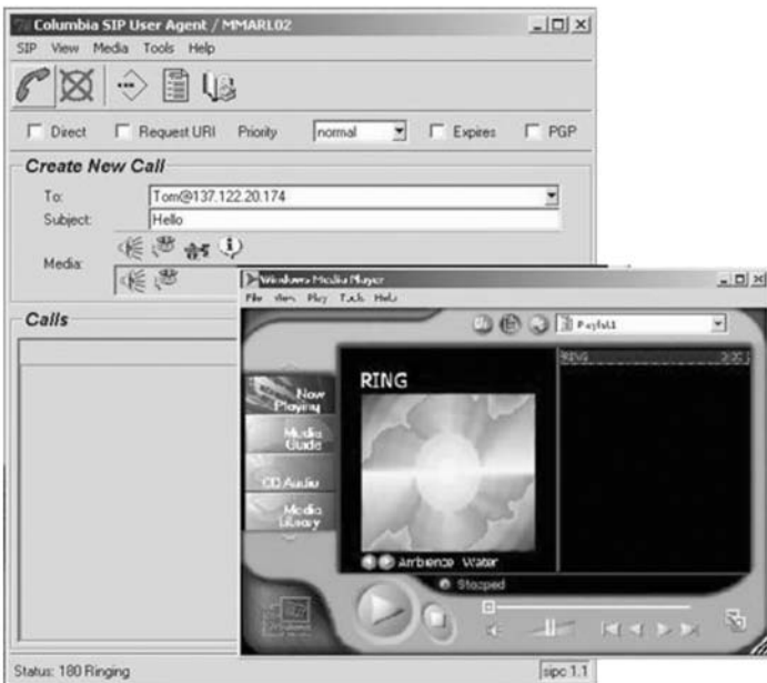
Figure 4.13 How a SIP call is initiated via the SIP user agent.
